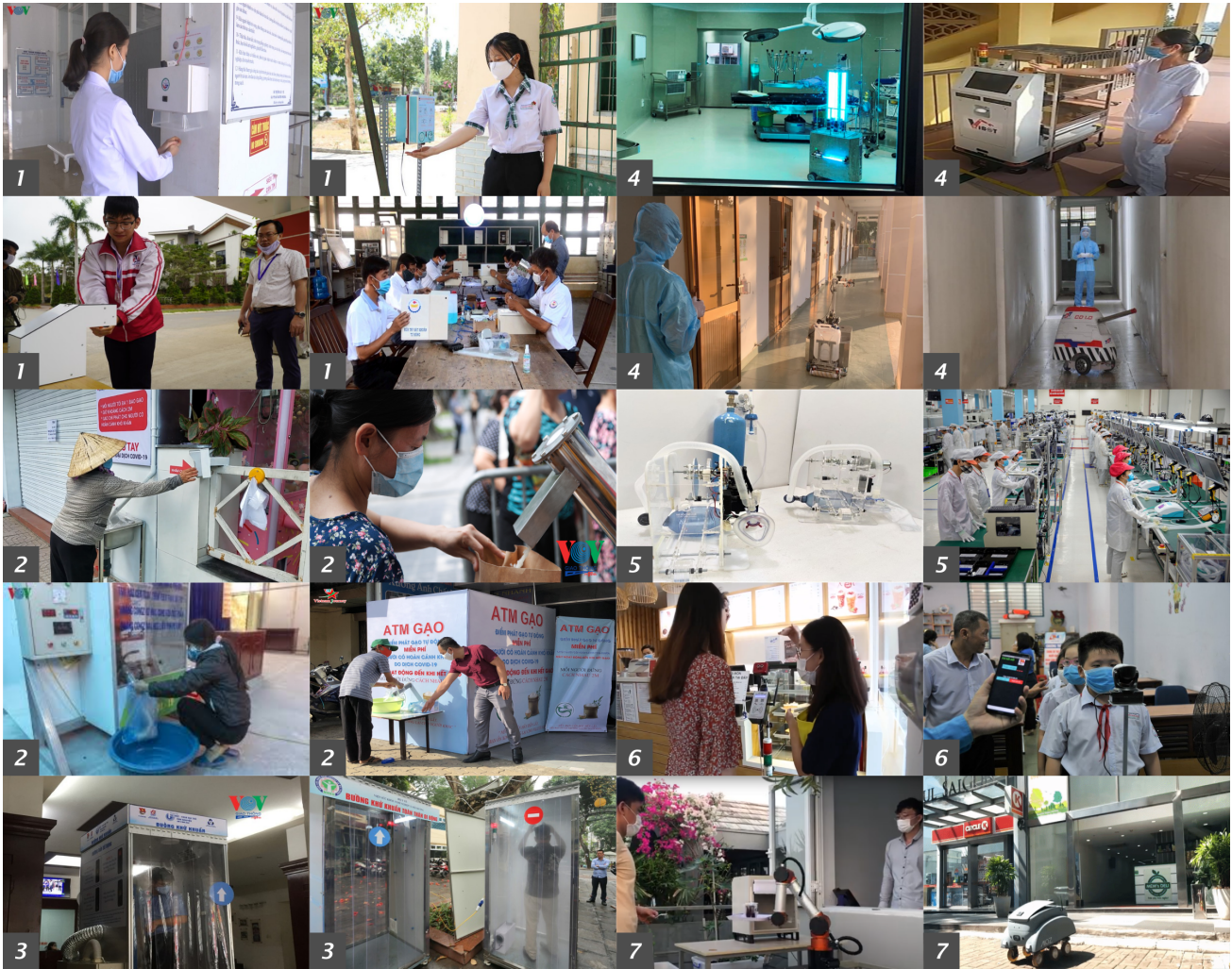
Figure 1: Localized automation solutions being deployed in Vietnam during the COVID-19 pandemic have been well-covered by the media. (1) Automatic hand sanitizer dispensers; (2) “Rice ATMs” (automatic rice dispensers); (3) Mobile disinfection chambers; (4) Mobile robots for disinfection, safe distribution, and communication; (5) Localized ventilators; (6) Automatic body temperature measurement system; (7) Others: a robot for safe takeaway services, a patrol robot. Credits: Solution developers, VOV, VTV, Thanhnien.
